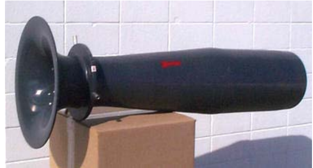
Diesel locomotive turbocharger flow meter 24.64" diameter with an 8.64" throat
