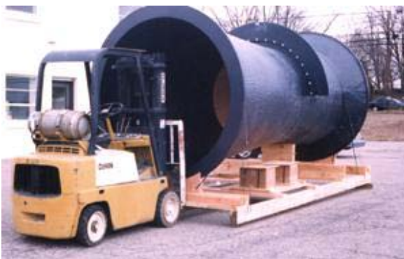
96" Vinyl ester fiberglass universal venturi tube manufactured by DECON for BIF.
