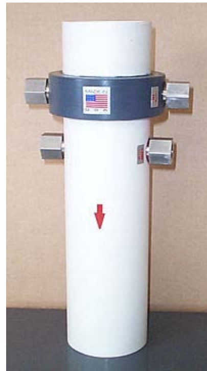
DVT-2300 PVC Venturi inserted in schedule 40 PVC pipe with 316 stainless steel pressure taps calibrated for air service by CEESI
